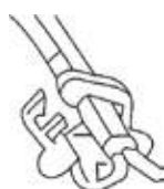
Insert cable in the ISOLATOP jaw
